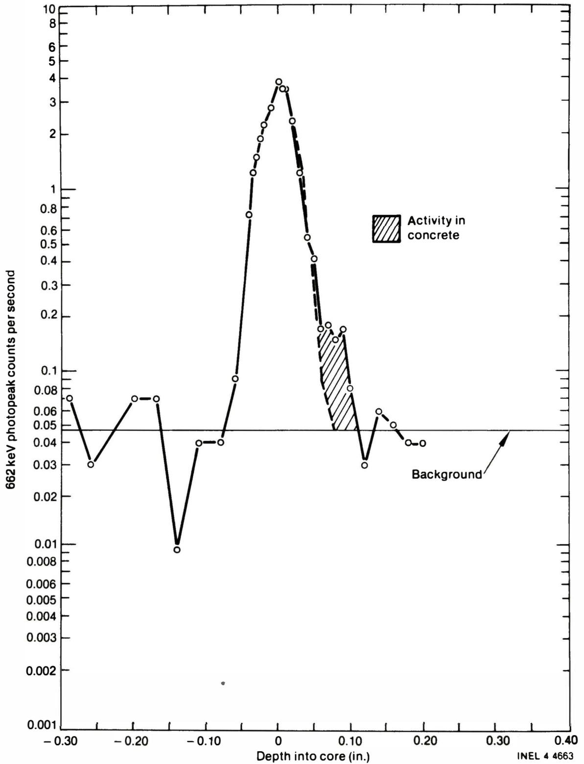
Figure 8.  $^{137}\text{Cs}$  distribution profile within concrete core sample number 347-5.
