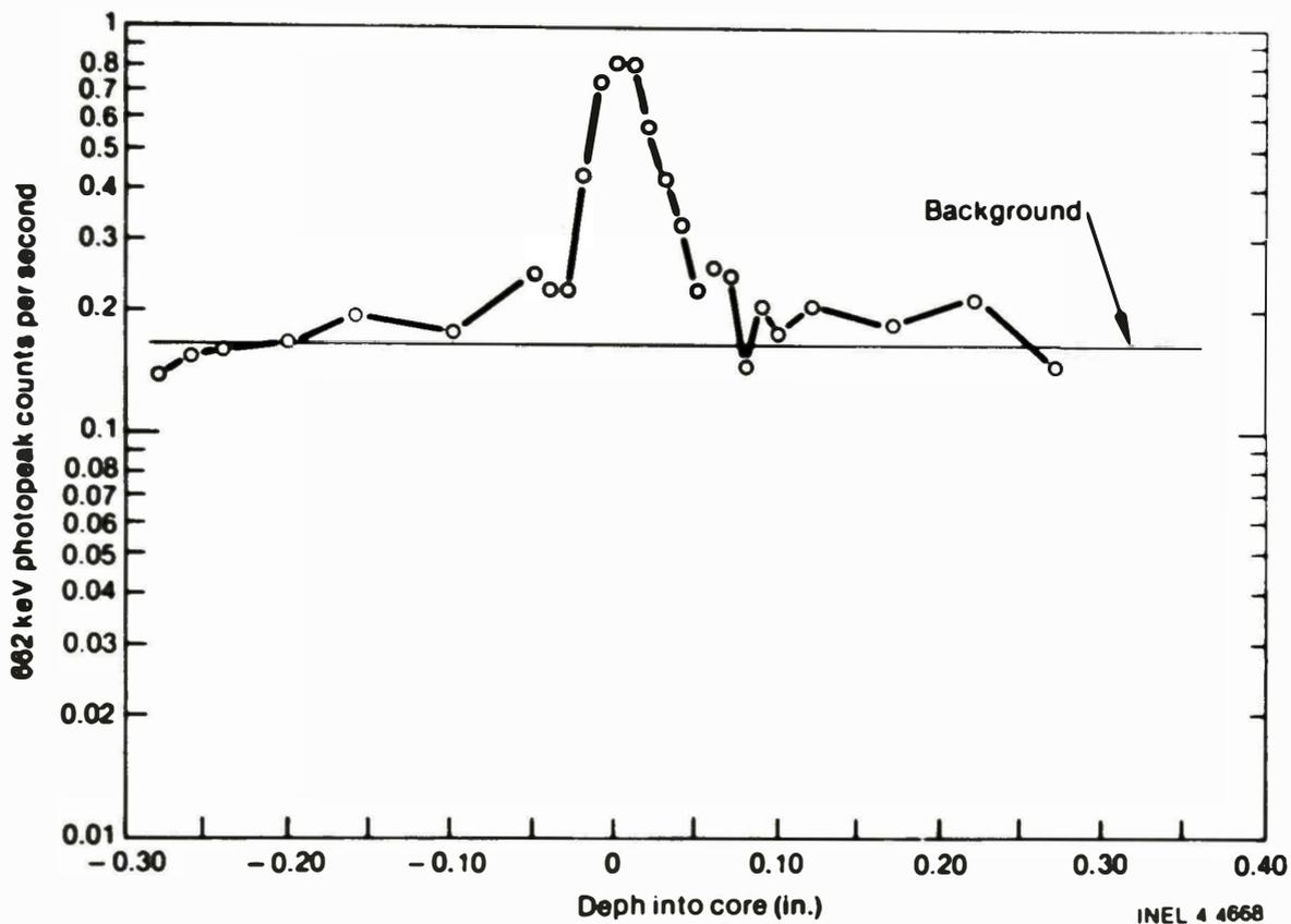
Figure 7. <sup>137</sup>Cs distribution profile within concrete core sample number 305-8.
